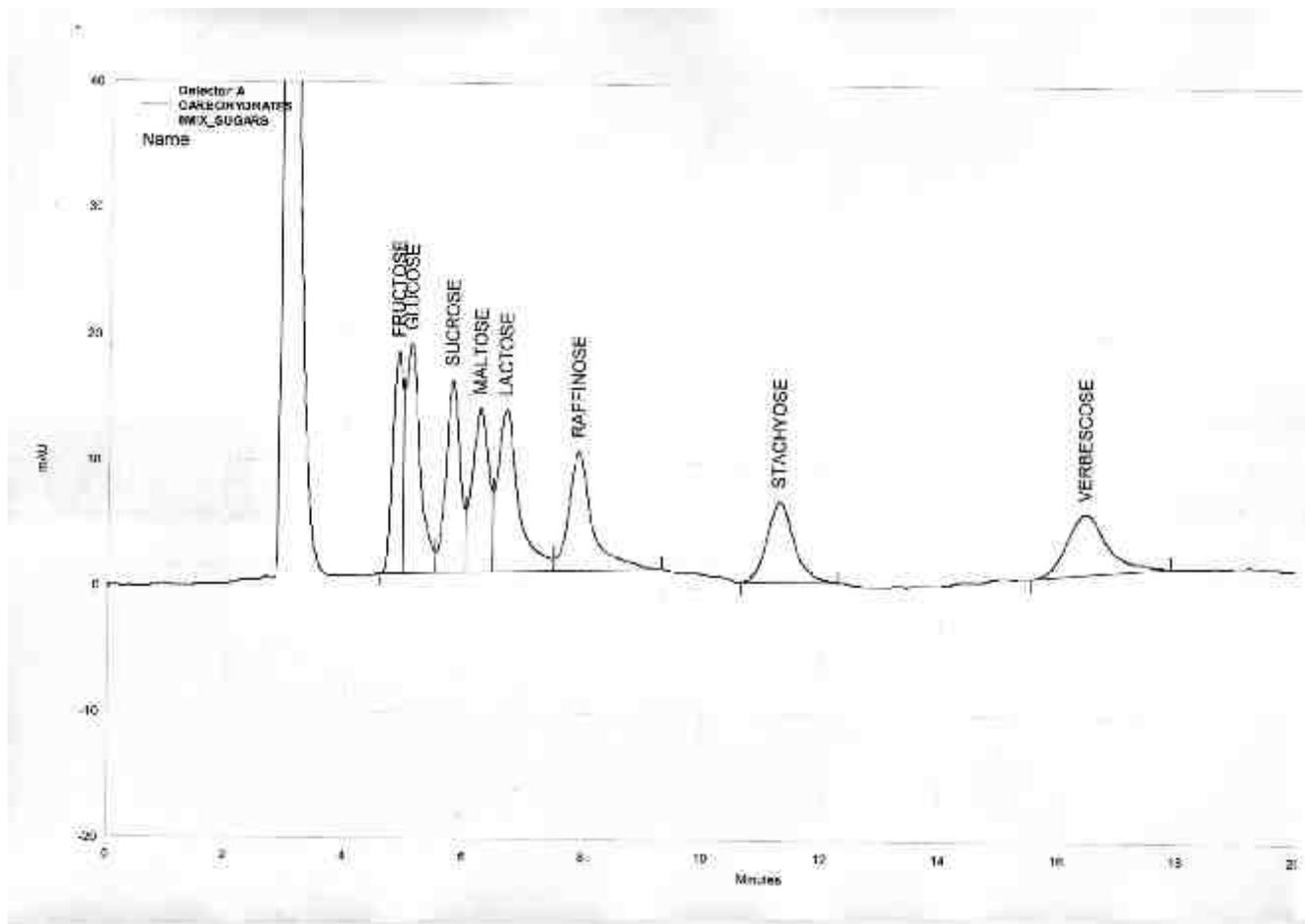
**Fig 2. Typical chromatogram of raffinose family sugars from green gram dhal extract**
